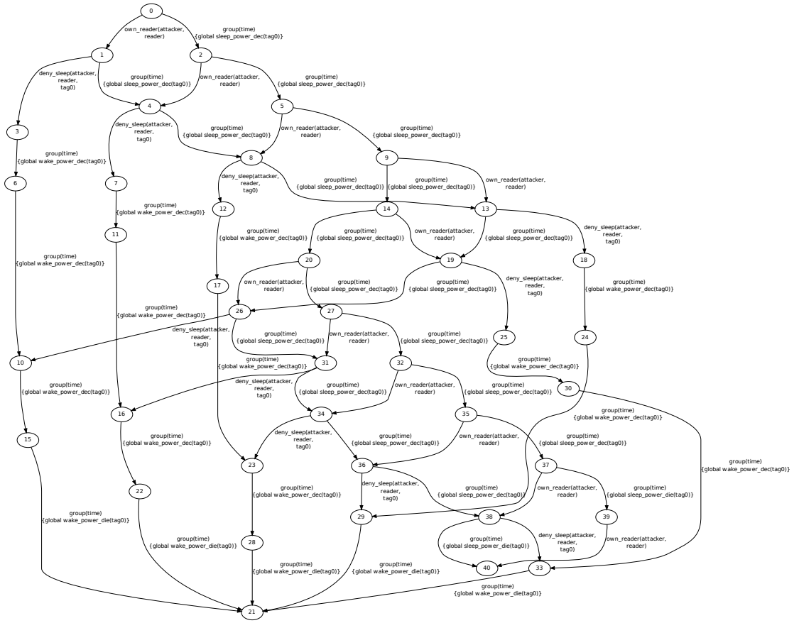
Figure 5.15: One tag RFID system attack graph (full depth)
